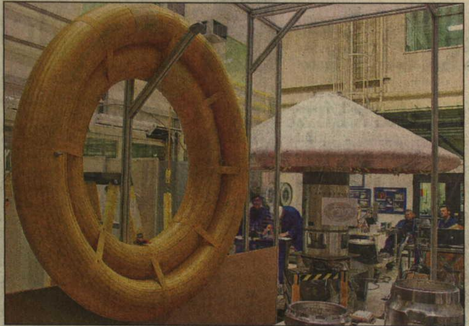
A hypersonic inflatable aerodynamic decelerator is shown in the background at the Nasa Langley research center in Hampton, Virginia. It is made up of high-tech fabric rings, similar to those seen in the foreground. The rings will be filled with nitrogen
